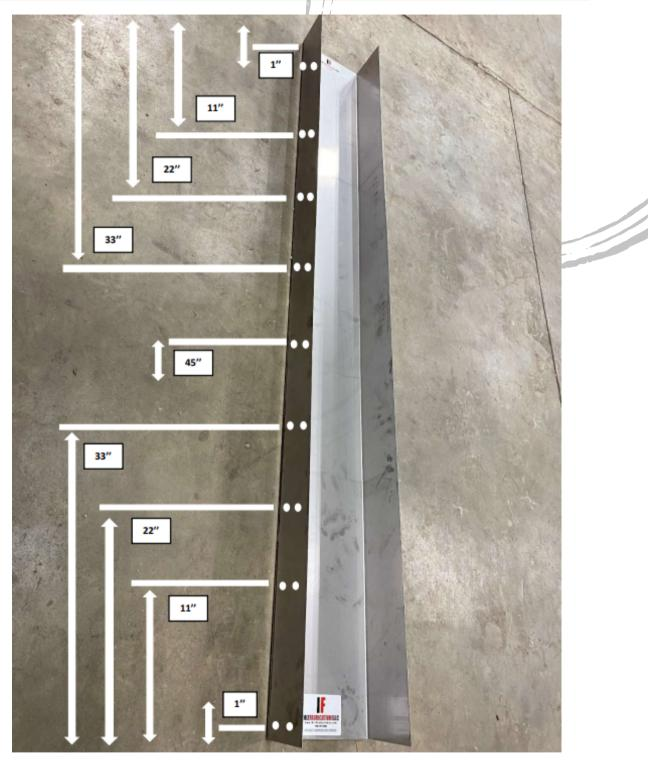
**NOTE:** Do **NOT** drill holes in the liner, this picture is just for reference where to drill the OEM elevator.
