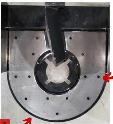
Clamp plate in place. Plug weld all provided holes to secure.
