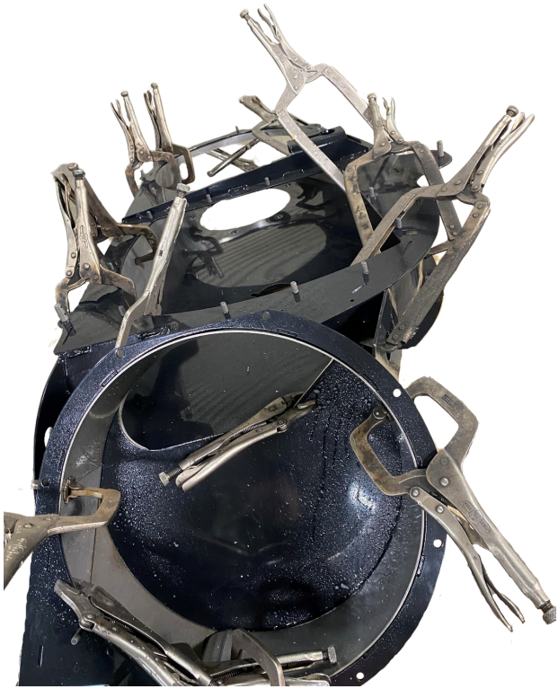
Liners clamped in place
